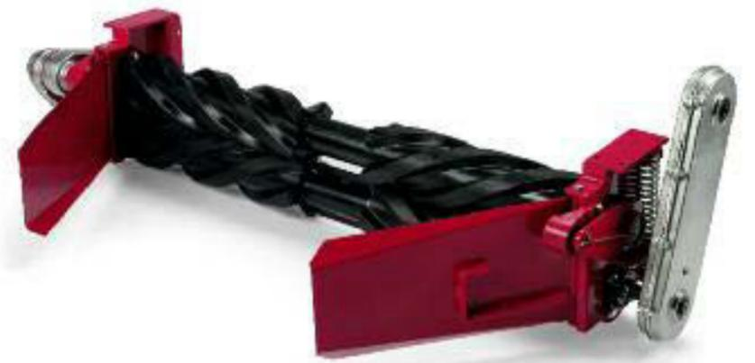
The job of the conditioner is to press and split the fodder; this opens the outer waxy layer of the stems, so that the excess water flows out, thus accelerating the drying process, while maintaining the body and all the nutritional elements.
