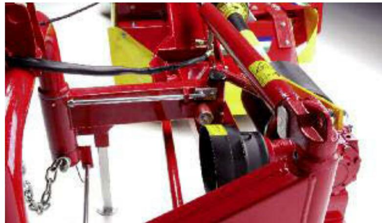
The 3 point hitch with swinging drawbar means the mower can adapt to any working condition: the dual movement enables the mower to adjust to the ground surface and the self adjusting compensation spring controls the cutterbar down pressure.
