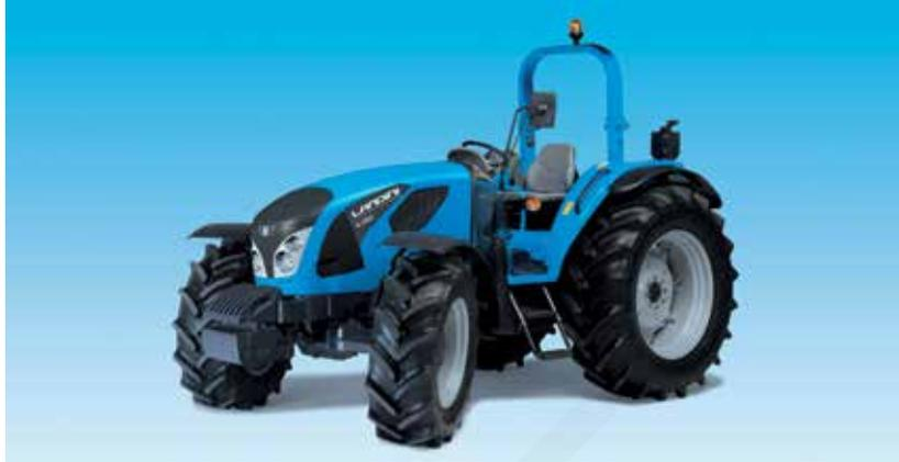
The 5H tractor range from Landini is revamped with the new Perkins 854E-E34TA 3.4L, four-cylinder engines, all featuring a two-valve cylinder head, a common rail injection system, turbocharging and an air-to-air aftercooling system. Equipped with an innovative exhaust gas recirculation system (EGR) which reduces NOx emissions at source, these engines meet the Tier 4 Interim emission regulations without the use of fuel additives.
